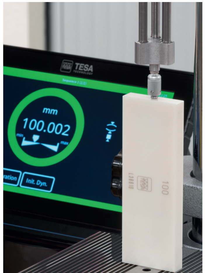
Checking of ceramic gauge block
