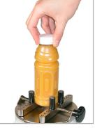
Higher capacity Series R53 torque sensors accommodate larger sample sizes, as shown in the beverage closure application above.
