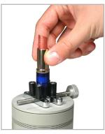
^ Low capacity Series R53 torque sensor is shown in a cosmetic packaging test.
