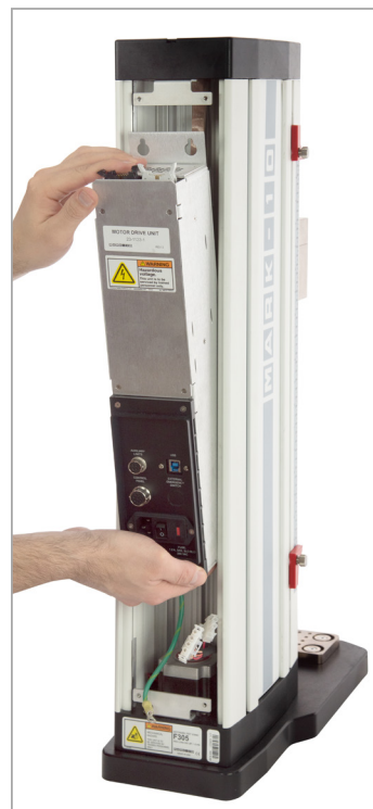
Removing the electronics module
