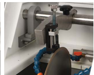
Wide range of specimen vises
