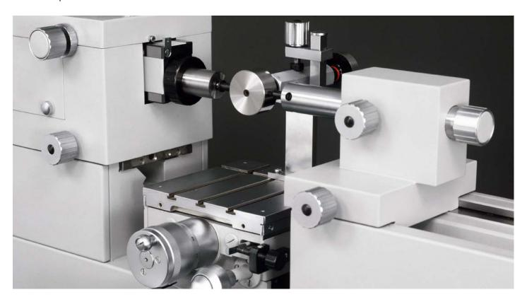
Thread gauge measurement: three wire method
