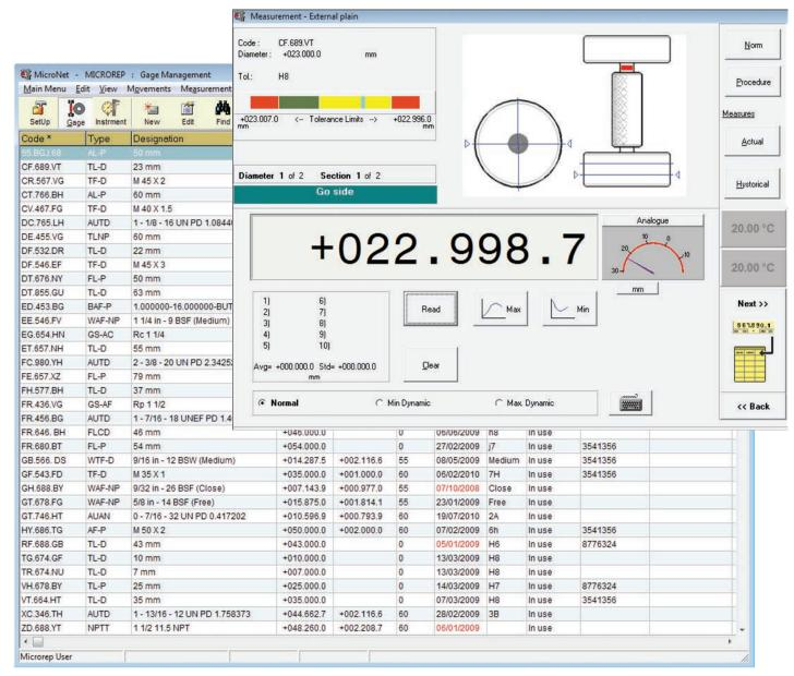
**Plug gauge measurement:** the movement of the work table enable high speed location of the inversion point
