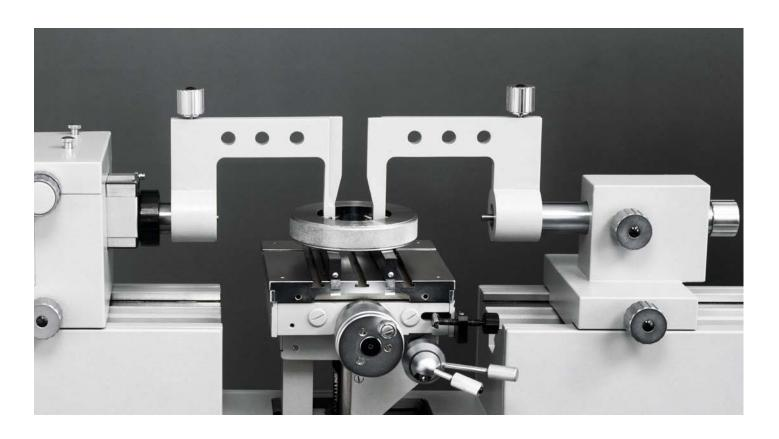
**Thread ring gauge measurement:** a pair of large contact arms and small contact arms, together with 12 pairs of spheres, are used to measure thread ring gauges
