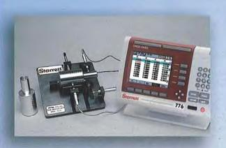
The 776 accepts multiple gage inputs simultaneously – invaluable for applications such as this Starrett special gage fixture
