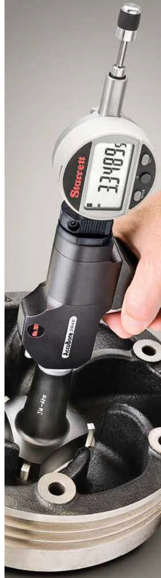
770BXTZ-250 Bore Gage with PT24272 Depth Stop Collar
